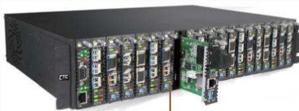
Chassis backplane consists of passive components
